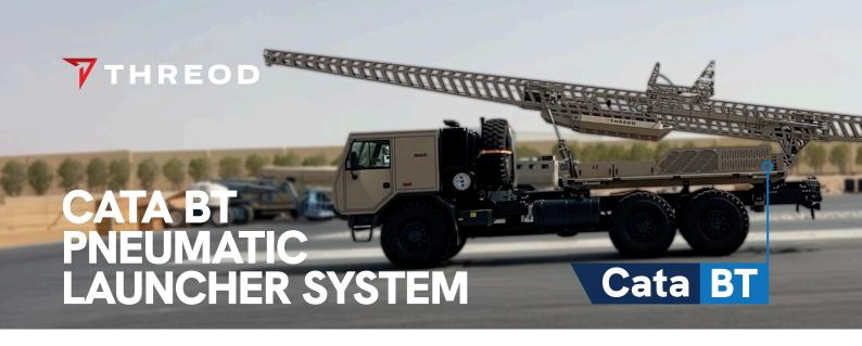
The Cata BT is a pneumatic launch system for the rapid deployment of one-way effectors and compatible with diverse all-terrain vehicles for enhanced mobility.
