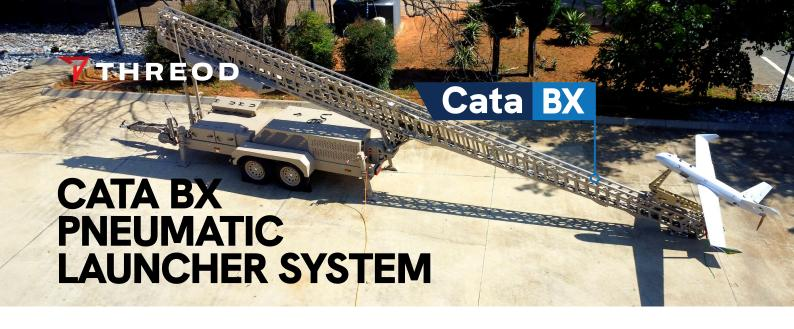
Cata BX is a pneumatic launcher system designed for rapid deployment of one-way effectors and target drones.
