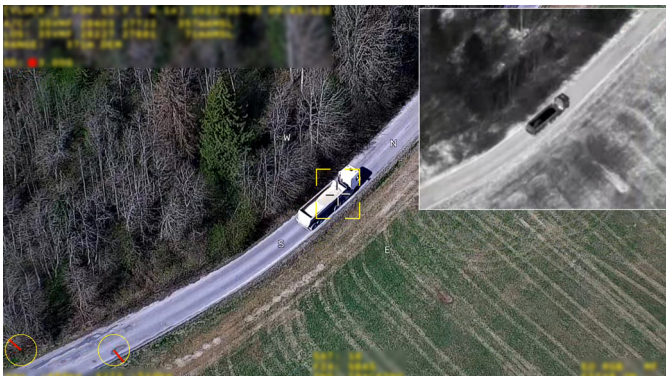
Picture-in-picture to see the target in both visible and thermal spectrum simultaneously
